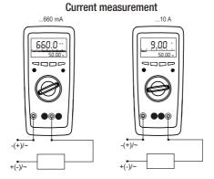
AC current measurement with (clip-on) current transformers
