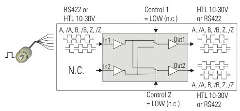
Input 1 is used as encoder input, and Input 2 remains unconnected. The input can be set to either symmetric (differential) format using A, /A, B, /B, Z, /Z channels, or to asymmetric (single-ended) format using A, B, Z channels only. Acceptable input levels are RS422, TTL and HTL 10 ... 30 V.
