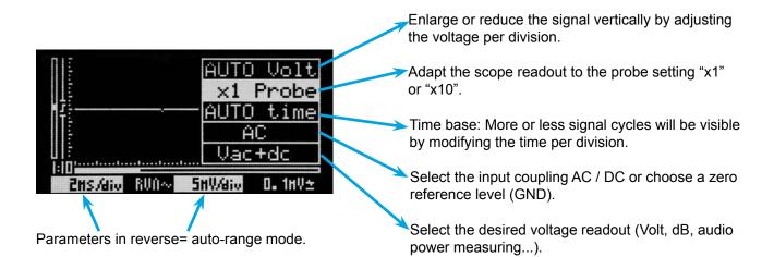
**Note:** The menu will exit automatically if no button is pressed for a few seconds, or exit by a long press on the menu button.
