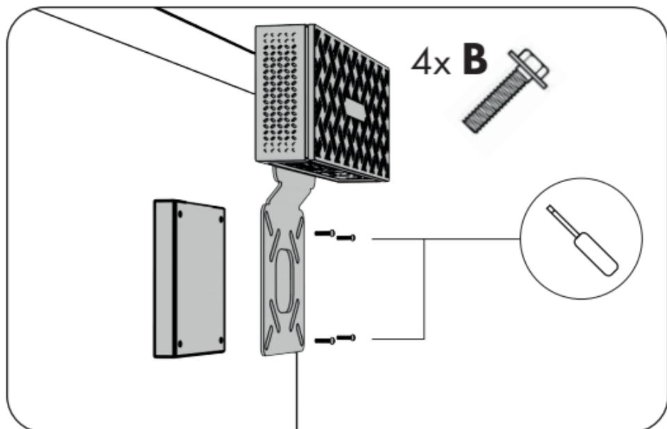
c. If you are using a monitor arm, position the unit between the VESA mount of the monitor and the VESA mount of the monitor arm as shown below and secure it using the four M4x12 mm screws provided.
