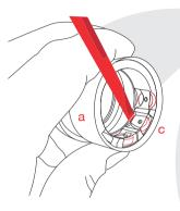
**3** Remove batteries with flat plastic tool
