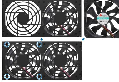
**b** Connect the 2 fan cables to the connectors located near the bottom of the fan socket, and then replace the fan panel.
