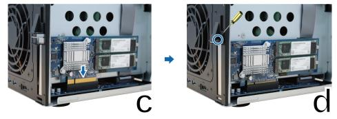
5 Put back the upper case removed in step 2 and tighten the srcews.
