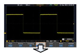
9. Press the relevant function key again to reduce the bottom menu. For example: press the Trigger Menu key to reduce the trigger menu.
