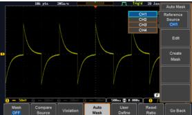
4. Press the *Edit* button from the side menu if you want to further adjust the mask pattern. Otherwise, go to step 9 below to create the mask directly without adjustment.
