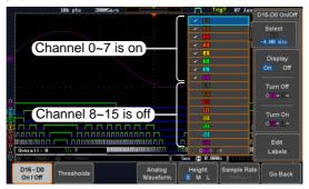
4. Press the *Display* soft-key or the *Select* key to toggle the selected channel or group on or off.
