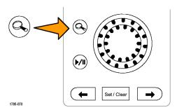
Examine the zoomed view of the waveform that appears on the larger, lower portion of the display. The upper portion of the display will show the position and size of the zoomed portion in the waveform, within the context of the overall record.
