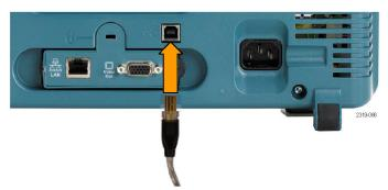
**NOTE.** The oscilloscope recognizes the printer only when the printer is powered on.
