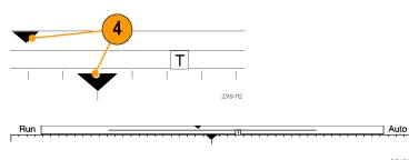
The waveform record view shows the trigger location relative to the waveform record. The line color corresponds to the selected waveform color.
