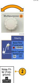
3. Push Glitch Capture Background to turn off the background waveform that contains the higher frequency components of the signal.
