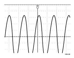
4. The expansion point icon (an orange triangle) shows the point that the horizontal scale expands and compresses around.
