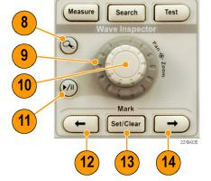
Play-pause button. Push to start or stop the automatic panning of a waveform. Control the speed and direction with the pan knob.
