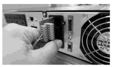
4. Connect the cable, then screw the cover as following pictures.
