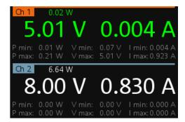
Figure 5-2: Channel display area for 3-channel and 2-channel instrument
