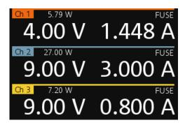
Figure 5-11: Fuse switched on for the respective channel
