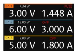
Figure 5-13: Indicator of OVP/OPP when tripped
