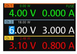
Figure 5-3: Color coding of operating condition
