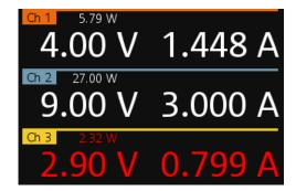
Figure 5-12: Output of Ch 3 in CV and CC mode
