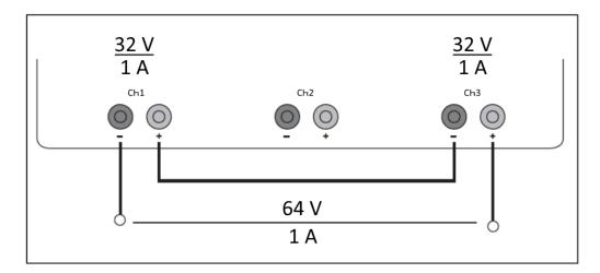
Figure 7-1: Example of serial connection
