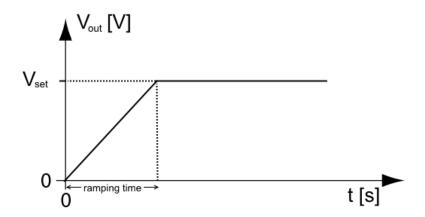
Figure 5-17: Ramping voltage output
