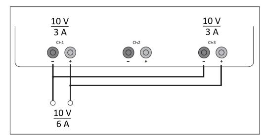
Figure 7-2: Example of parallel connection
