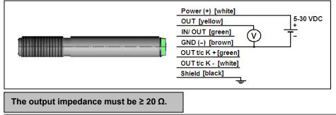
On the model CSTCLT15 you can choose between a mV output (0-5 or 0-10 V; scalable via software) and a thermocouple output type K.
