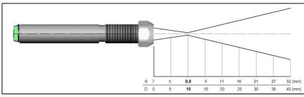
Optical chart CS (15:1) with CF-lens (0,8 mm@ 10 mm)
