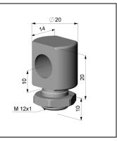
Mounting bolt with M12x1 thread, adjustable in one axis [ACCTMB]
