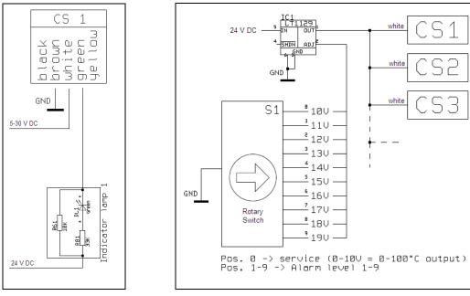
Open collector output for direct 24V DC signal lamp control Common power supply voltage change to adjust simultaneously alarm levels and emissivity values [Vcc adjust mode]
