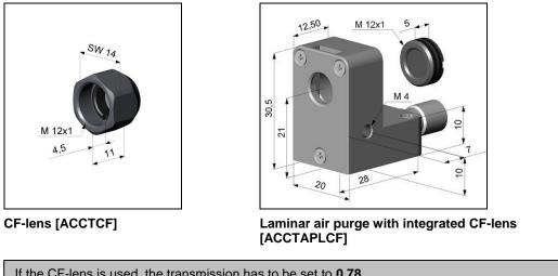
If the CF-lens is used, the transmission has to be set to **0,78**. To change this value the optional USB-Kit (including CompactConnect software) is necessary.
