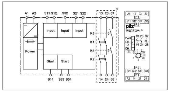
\*Insulation between the non-marked area and the relay contacts: Basic insulation (overvoltage category III), Protective separation (overvoltage category II)
