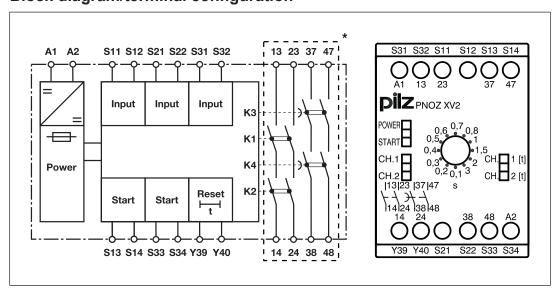
\*Insulation between the non-marked area and the relay contacts: Basic insulation (over-voltage category III), Protective separation (overvoltage category II)
