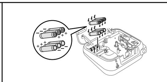
Insert six new AAA alkaline batteries (LR03) or fully charged Ni-MH batteries (HR03), making sure that their poles point in the correct directions.
