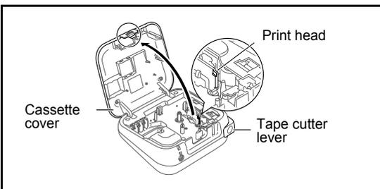
Open the cassette cover by pressing the above indicated area at the top end of the machine.
