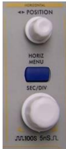
Fig. 9 Horizontal Control Zone
