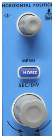
Fig. 12 Horizontal Control Zone
