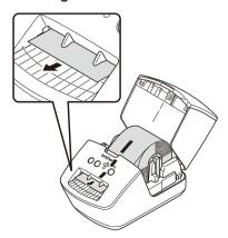
• Push the first label through the Label Output Slot until the end comes out of the Slot as shown.
