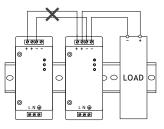
Parallel Operation A (Unable to use) Parallel Operation B (Unable to use)
