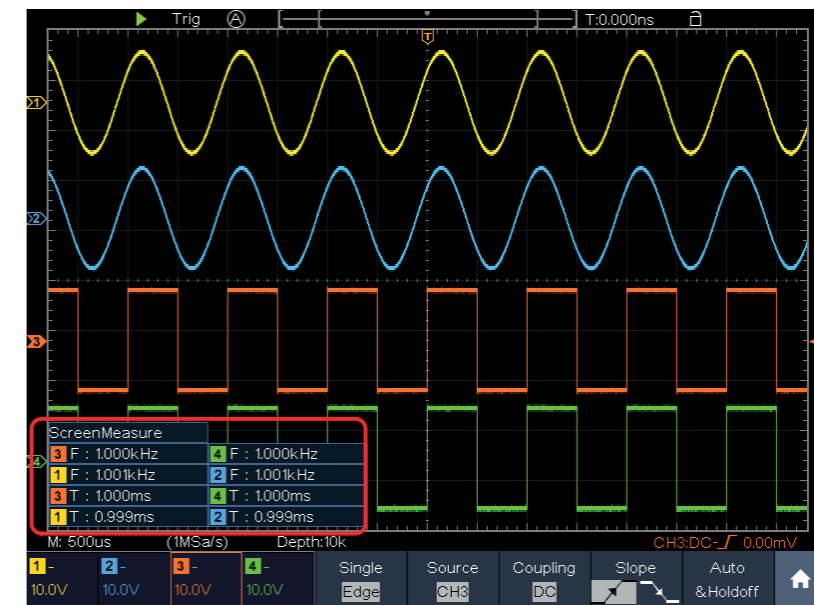
Figure 9-1 Measure period and frequency value for a given signal
