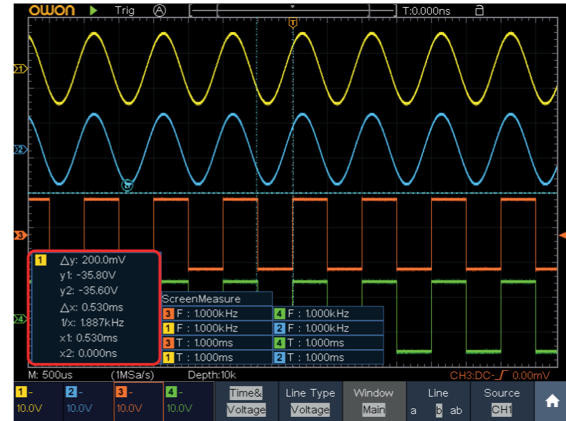
Figure 4-26 Time&Voltage Cursor Measurement
