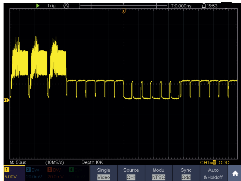
Figure 9-7 Waveform Captured from Video Field Trigger
