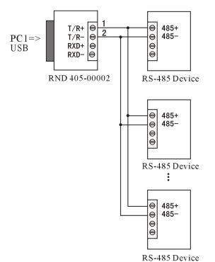
3.Half-duplex communication connection between RND 405-00002 interface converters
