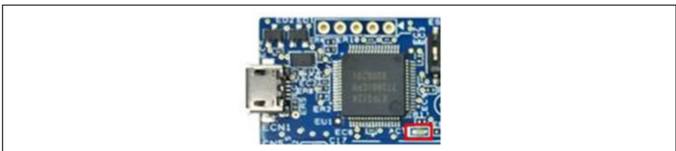
Figure 10. ACT LED on EK-RA4W1 Board
