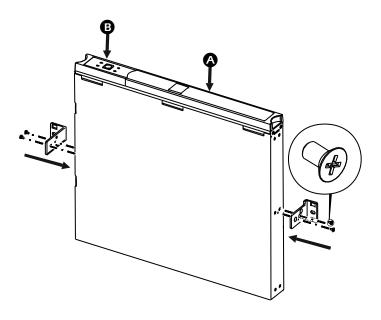
Note: Whenever possible, attach two screws into wall studs. If stud mounting is not possible, use an expandable wall anchor. Hardware is not included; 0.25 inch x 2 inch lag bolts are recommended.
