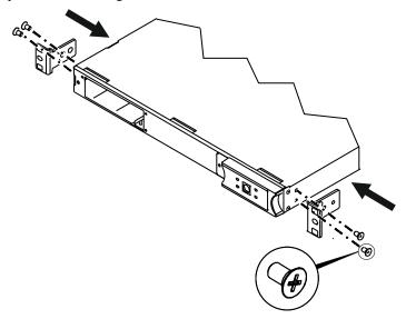
**6** Secure clip nuts to the rack, and attach brackets with provided screws.
