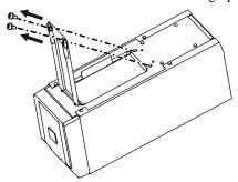
2 Connect black wire to battery (Red wire is already connected). **Note**: Small sparks at the point of battery connection are normal.
