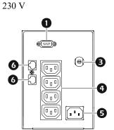
The top off-white outlet helps to provide surge protection only. Equipment plugged into this 500 VA outlet should require surge protection, but should not require power during a utility power outage. The lower three outlets help to provide battery backup protection, as well as protection from surges.
