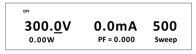
2. Press the On/Off key to enable (ON) the output and allow the sweep to run. The Enter key will begin to blink while the sweep is running.
