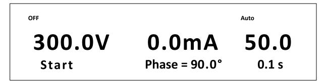
Use the numeric keys to set the start phase angle and press Enter to confirm the start phase setting. The following screen will be shown next.
