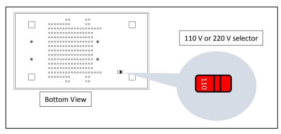
Figure 11 – Line Voltage Selector Location 9801
