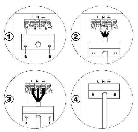
Figure 16 - AC Input Connection
