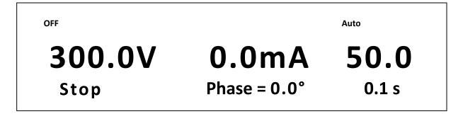
Use the numeric keys to set the stop phase angle and press Enter to confirm the stop phase setting.
