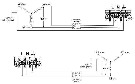
Figure 17 - Single Phase Mains Connection
