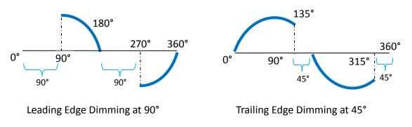
Figure 24 – Leading and Trailing Edge Dimming
