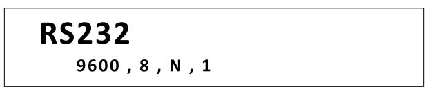
3. 9600 is the baudrate; 8 is the data bits; N is the parity; 1 is the stop bit.
