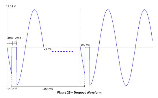
To create the waveform above, access the list mode as described *above* and enter the following parameters in the list mode file.
