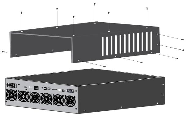
Figure 14 - Removing top cover
