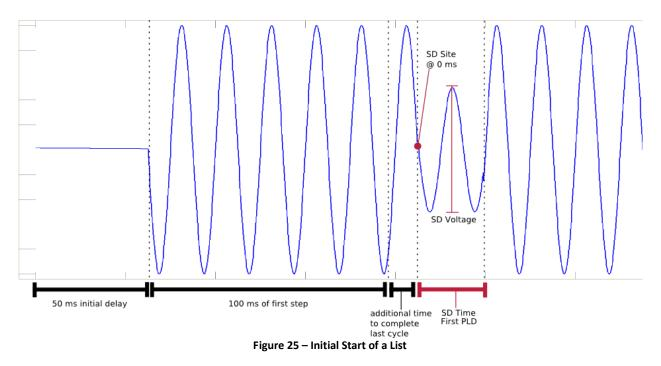
**SD Voltage** - This parameter defines the voltage level of the PLD.
