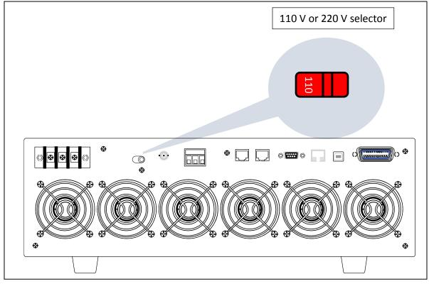
Use the line voltage selector on the rear panel of the 9803 and 9805 to set the input voltage of the instrument between 110 V and 220 V.
