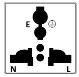
Figure 18 – Universal AC Output Socket
