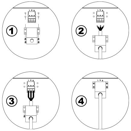
Figure 21 - Rear Panel Terminal Block Connection
