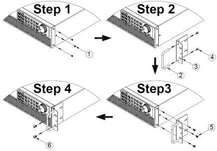
Figure 2.3 - Rack Mount Bracket Assembly
