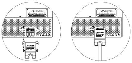
Figure 2.1 – AC Power Connection Diagram
