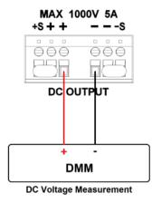
Figure 5.1 - Voltage Calibration Diagram
