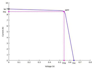
Figure 3.11 - PV Simulation Curve
