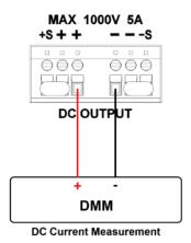
Figure 5.2 - Current Calibration Diagram
