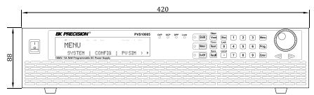
Figure 1.1 - Front Panel Dimensions
