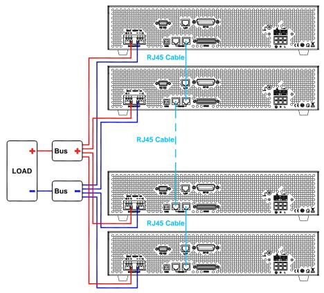
Figure 3.10 - Parallel Connection Diagram
