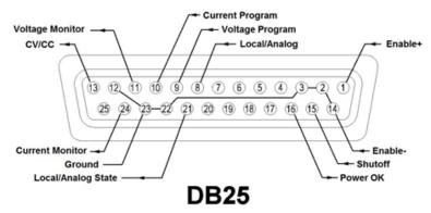
Figure 3.3 - DB25 Pinout
