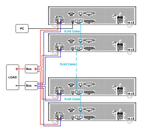
Figure 4.1 - RS-485 Connection Diagram for 10+ Units
