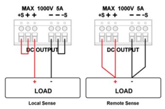
Figure 3.1 - Local/Remote Sense Connection Diagram
