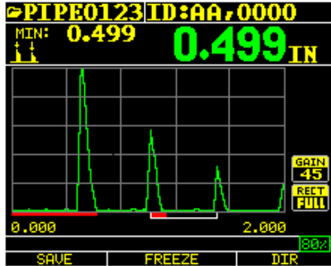
Example of Echo-to-Echo with blanking
