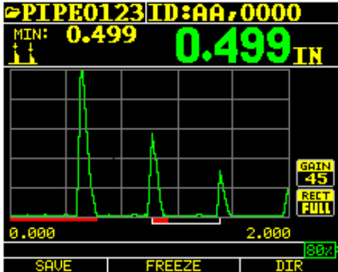
Color Waveform in Echo-to-Echo, filename, id, minimum, large thickness value, Echo-to-Echo, range, echoes, blanking, gain, rectification, battery life, save, freeze and directory.
