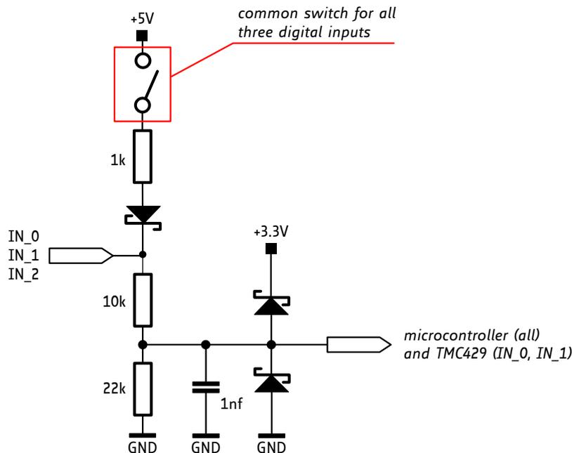
**Figure 3.5 General purpose inputs (simplified input circuit)**
