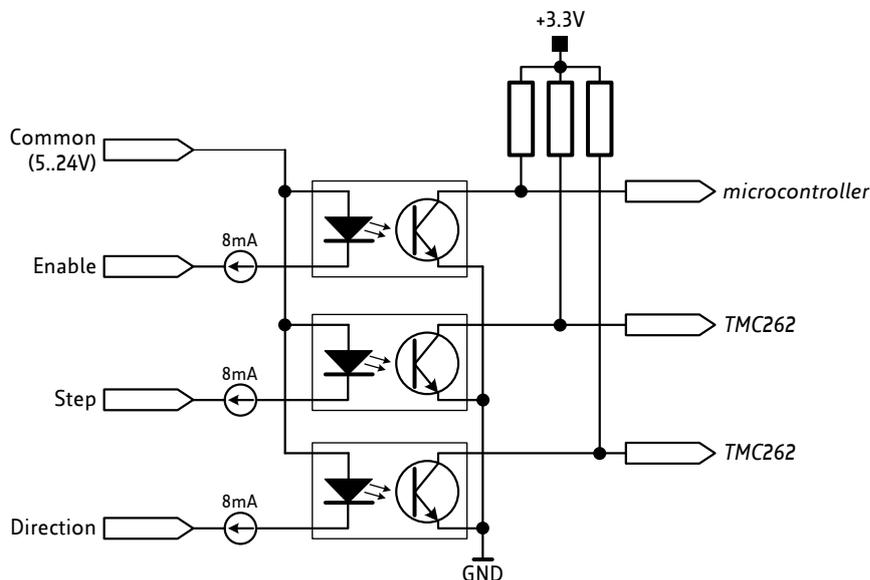
Figure 3.8 Step/Dir/Enable inputs
