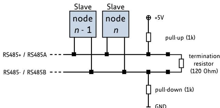
Figure 3.4 Bus lines with resistor network
