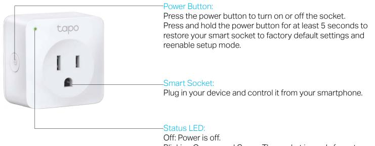
Off: Power is off. Blinking Orange and Green: The socket is ready for setup. Green: The socket is working normally. Blinking Green: The system is being upgraded. Orange: There is an error. Blinking Orange: The socket is connecting to a Wi-Fi network.
