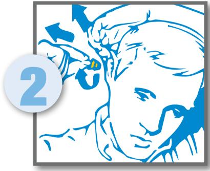
Insert it into the ear canal with a gentle twisting and turning motion until a good seal is obtained.
