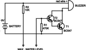
T1 & T2 are configured as a Darlington switch hence only a very small current is needed to make T1 conduct and activate the alarm sound.
