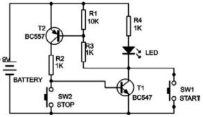
R2. T1 also starts to conduct. From this point on, both transistors keep each other in conducting state, even when the "START" button is released. Pressing the "STOP" button will end the current flow towards the base of T1 and it will stop conducting. The circuit is interrupted and T2 will also stop conducting. The LED will turn off.
