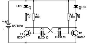
The LED on-time can be calculated: T = 0,693 x R1( $\Omega$ ) x C1 (F) T = 0,693 x 100.000 x 0.00001 = 0,693sec.
