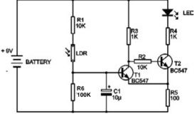
via R2 and R3 and conducts; the LED will be on. When light shines on the LDR the voltage on the base of T1 rises. T1 will start to conduct when this voltage is higher than the voltage over R5 +  $U_{be}$  of T1. When this is the case, the base voltage of T2 drops and T2 does not longer conduct and the LED goes off. Because of the change in flow through R5 when the LED switches off, the threshold level for which T2 will conduct again in darkness also changes.
