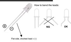
A LED is a Light Emitting Diode, it can emit light using a small current (max 20mA with a 1.8V drop). Watch the polarity, long lead = + ! (Velleman part# L-7104LGD & L-7104LID)
