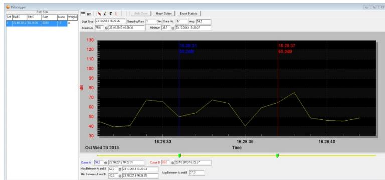
The measurement series available in the instrument memory are displayed on the left-hand side and can be selected by clicking on them with the mouse.
