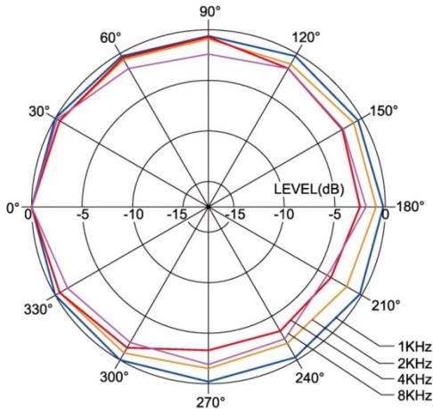
**Directional characteristics of the sound level meter**
