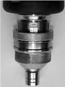
To set the torque, screw on or unscrew the lock nut. Then the removing steel ring can be fixed by a grain \* taking care of it in the appropriate grooves.
