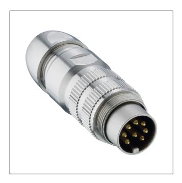
Next Generation – Plug acc. to AISG specification and IEC 61076-2-106, IP68, with threaded joint, vibration protection and solder terminals, 360° shielded, optimized assembly
