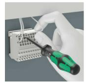
The blade tip stays in the terminal block, leaving both hands free to insert the end of the wire.
