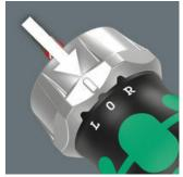
The ratchet mechanism is finetoothed for a low return angle. The screwdriving directions right/fixed/left can be set with the reversible ring. The magnetic bit mounting is suitable for bits with 1/4" external hexagon drive as per DIN ISO 1173-C 6.3 and Wera connection series 1
