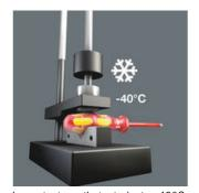
Impact strength tested at  $-40^{\circ}$ C, guaranteeing safety even under extreme conditions.
