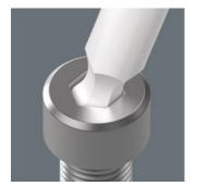
The spherical drive profile means that it is possible to swivel the axis of the tool to that of the screw, and therefore enable angled, "around-the-corner" screwdriving
