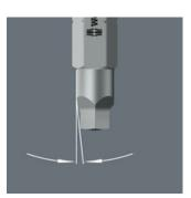
V bits have a conical profile. The clamping forces thus resulting hold Robertson screws securely on the tip of the tool. Ideal for screwdriving at difficult-to-access places.
