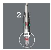
Higher peak loads are minimised through the torsion effect of the bit shaft (Phase 2). This effect is achieved with a specific heat treatment after the hardening process of the bits. This reduces the hardness of the shaft in comparison to the drive tip.
