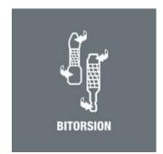
Peak forces that occur in power tool applications often result in premature wear of bits or damage to the screw head. This usually occurs during initial power-up and the when the screw comes to a standstill. Screwdriving could become more productive and safer if these peak loads could be minimised. The Wera BiTorsion system prevents premature wear. The service life of the tool is extended and the productivity of power applications tool significantly increased.
