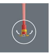
The two gripper arms spread further apart as they are pushed against the surface and automatically snap back when the head of the screw is countersunk.
