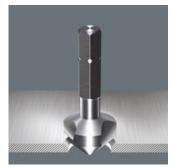
3-flute countersink bits, 90° • Application: Deburring, chamfering and countersinking • 1/4" drive suitable for holders as per DIN 3126-D 6.3 (ISO 1173) • Hexagon shaft for very high torque transfer • HSS = high speed steel • Finely adjusted material elasticity for long service life • 3 tips • Excellent centring properties • Straightforward cutting • Perfect chip removal • Low jamming risk • Precise return control • High corrosion protection
