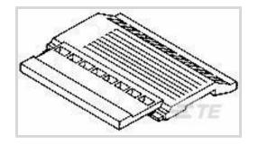
Number of Positions: 26 Centerline (Pitch): 2.54 mm [.1 in] Primary Product Material: Thermoplastic Product Profile: Low Connector Cover Type: Polarizing
