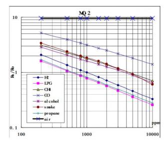
According to the figure, we can see that the minimum concentration we can test is 100ppm and the maximum is 10000ppm, in a other word, we can get a concentration of gas between 0.01% and 1%. However, we can't provide a formula because the relation between ratio and concentration is nonlinear.
