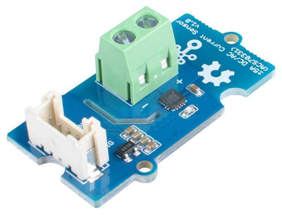
The Grove - ±5A DC/AC Current Sensor (ACS70331) is a high precision DC/AC current sensor based on ACS70331. The ACS70331EESATR-005B3 is Allegro's high sensitivity, current sensor IC for <5 A current sensing applications. It incorporates giant magneto-resistive (GMR) technology that is 25 times more sensitive than traditional Hall-effect sensors to sense the magnetic field generated by the current flowing through the low resistance, integrated primary conductor.
