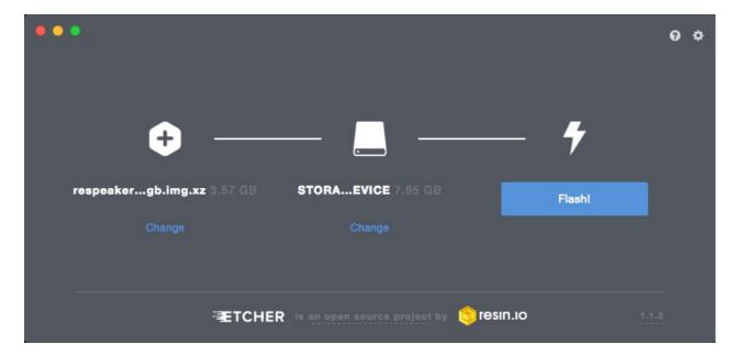
• Step 4. After writing the image to the SD card, insert the SD card in your ReSpeaker Core V2. Pow er the board using the PWR\_IN micro usb port and DO NOT remove the SD card after powering on. ReSpeaker Core V2 will boot from the SD card, and you can see USER1 and USER2 LEDs light up. USER1 is typically configured at boot to blink in a heartbeat pattern and USER2 is typically configured at boot to light during SD card accesses. Now, you should go to the next part: Serial Console.
