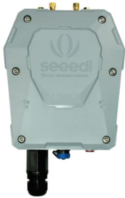
① LoRaWAN Gateway
