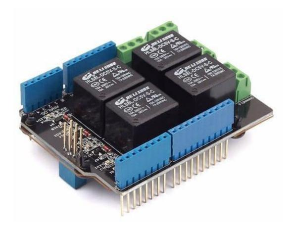
The Relay Shield provides four high quality relays that can control high current loads to Arduino / Seeeduino boards. It also provides NO (Normally Open) / NC (Normally Closed) contacts. A nice solution for controlling devices that cannot be directly controlled by Arduino's Digital I/Os. Standardized shield form factor enables smooth connection with Arduino and compatibles. The shield also has four LED indicators to show the on/off state of each relay.
