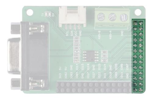
We use a 2X13 Female Header to plug this module into the Raspberry Pi, please make sure the pins are aligned.
