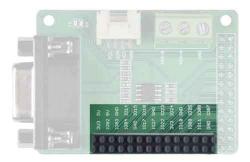
This RS-485 Shield occupies 26 Raspberry Pi pins, and only 5 GPIO pins are actually used. We take these 26 pins out in case you need those pins for other purposes.
