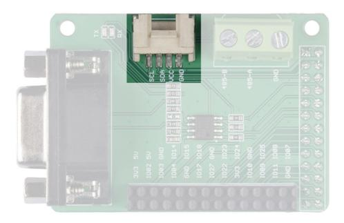
We have reserved the I2C interface so that you can easily use it with I2C devices. It should be noted that the VCC of this port is 5V, you need to confirm that whether the module is compatible with 5V voltage.
