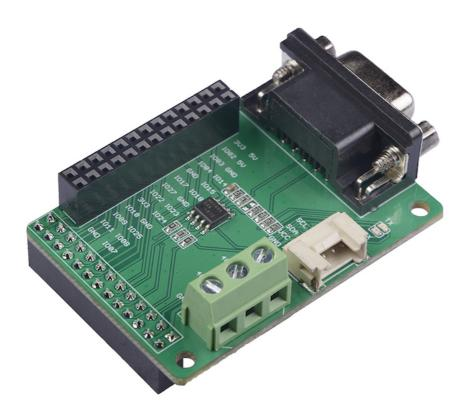
RS-485 is a cost-effective solution in serial communication networks. It can be used up to data rates at 10 Mbit/s or distances up to 1200m at lower speeds. This RS-485 Shield is a standard add-on board for Raspberry Pi. It is integrated with simple screw terminal as well as DB9 interface.
