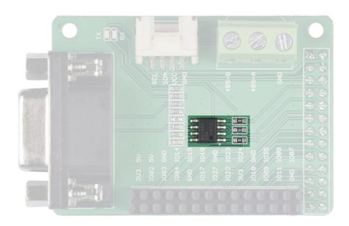
We use the MAX485ESA IC for this shield, for more detail about this IC, please check the MAX485 Datasheet
