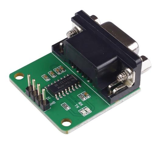
Most of the MCUs use TTL levels, and the computer serial port generally uses 232 levels. If we want the computer to communicate with the MCU, we need this **RS-232 To TTL Conveter (MAX3232IDR)**.
